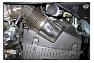
7. Loosen the hose clamp which secures the intake hose to the throttle body and remove the air box mounting bolt.
