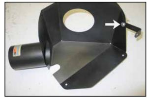
19. Install the heat shield mounting bracket (010051) onto the heat shield as shown using the provided hardware.
