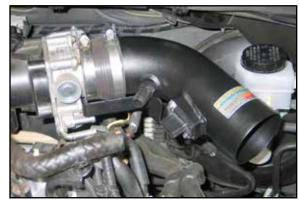
18. Install the K&N<sup>®</sup> intake tube into the silicone hose at the throttle body and align with the mounting bracket. Secure with the provided hardware and hose clamp.
