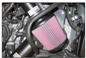
25. Install the K&N® air filter onto the K&N® intake tube and secure with the provided hose clamp. NOTE: Drycharger® air filter wrap; part # RU-4990DK is available to purchase separately. To learn more about Drycharger® filter wraps or look up color availability please visit http://www.knfilters.com®.
