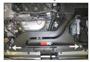
5. Remove the fresh air inlet assembly from the air box and radiator core support.
