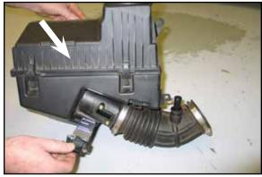
16. Remove the two bolts which secure the mass sensor to the intake tube and remove the mass air sensor as shown.
