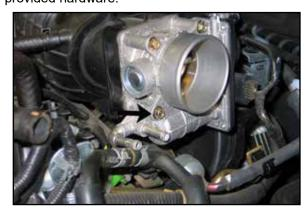
12. Remove the lower-front throttle body mounting bolt.
