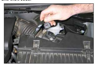
2. Disconnect the mass air sensor electrical connection and then unhook the wiring harness clips from the air box.
