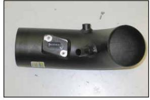
17. Install the mass air sensor into the K&N® intake tube and secure with the provided hardware.
