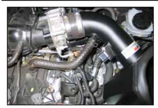
23. Install the factory crank case vent hose to the 1/4" npt vent installed onto the K&N® intake tube.
