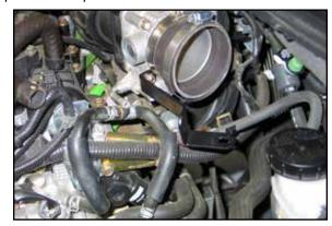
14. Install the provided silicone hose (084036) onto the throttle body and secure with the provided hose clamp.
