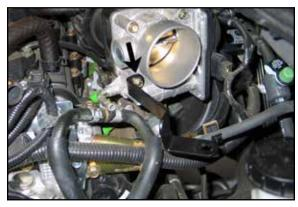
13. Install the tube mounting bracket (070091) onto the throttle body using the bolt removed in the previous step.
