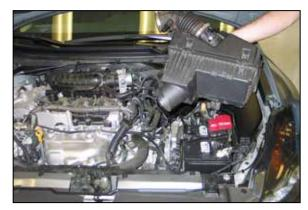
8. Remove the air box assembly from the vehicle. NOTE: K&N Engineering, Inc., recommends that customers do not discard factory air intake.
