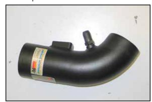
15. Install the provided ½"npt vent fitting into the K&N® Intake Tube as shown.
