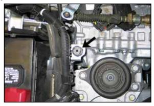
10. Install the 1.0" high rubber mounted stud onto the front air box mounting location using the provided hardware.
