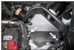
21. Install the heat shield into the vehicle so the mounting holes line up with the rubber mounted studs installed earlier. Secure the heat shield and mounting bracket with the hardware provided.
