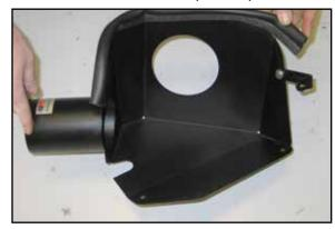
20. Install the provided edge trim onto the heat shield as shown.
