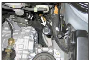
11. Install the ½" high rubber mounted stud onto the rear air box mounting location using the provided hardware.
